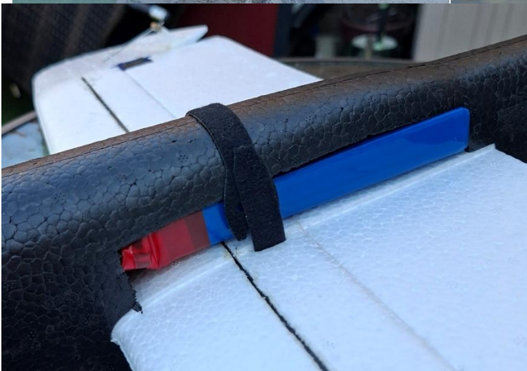
Above Three pics; Show battery mounted under wing, with Velcro strap holding it all together.
