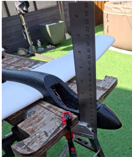
Above; Using workmate, bits of foam, set square and clamp, attempt to set up thrust line, and saw off nose.
