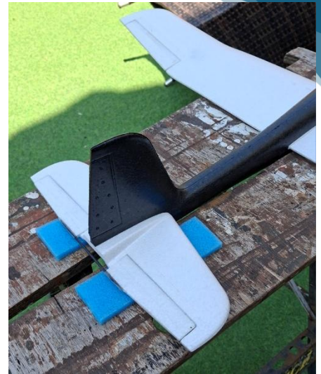
Above; Using workmate, bits of foam, set square and clamp, attempt to set up thrust line, and saw off nose.
