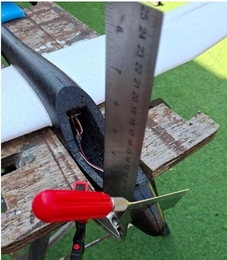
Above; Using workmate, bits of foam, set square and clamp, attempt to set up thrust line, and saw off nose.
