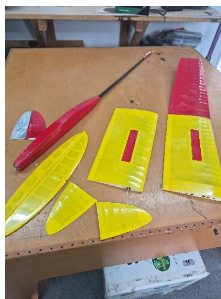
Peter Glassey's Apex AUW 442g CG came out at the centre of the range at 69.5mm
