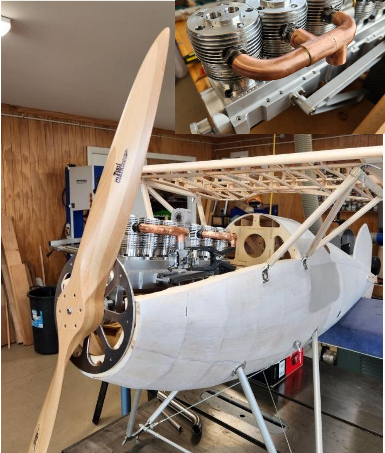
Above; 4. Trial fitting of the Engine in the fuselage of Russ's Albatross
