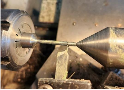
Left; Machining the E clip groove, 0.6mm by 0.4 deep. Right; Completed Inlet and Exhaust valves
