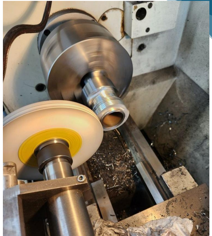
3. Grinding the top of the cylinder liner
