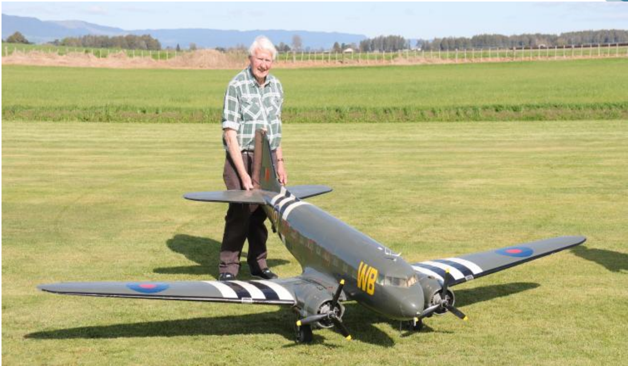
Dennis Clark's 1/8 scale DC3. It has a lot of detail, with thin aluminium covering showing countless rivets. This model was certified way back in 1993 but had not been flown again until recently, with Colin Austen demonstrating it very nicely at the rally. It was also great to see Colin's own venerable Beech C18 (twin Zenoah 62s) being flown again.
