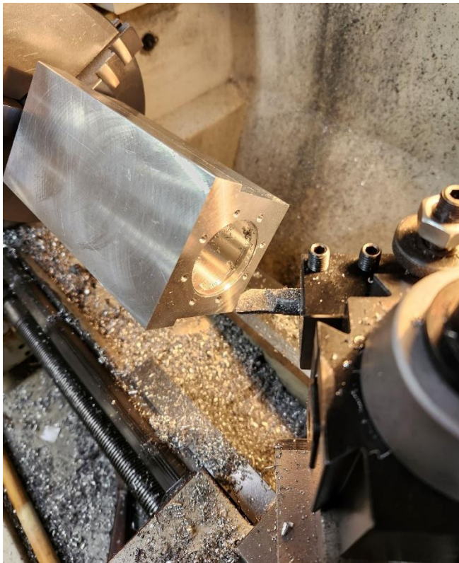
Crankcase in lathe, note 2kg lead balance weight.
