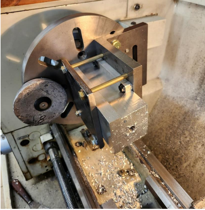
Crankcase in lathe, note 2kg lead balance weight.
