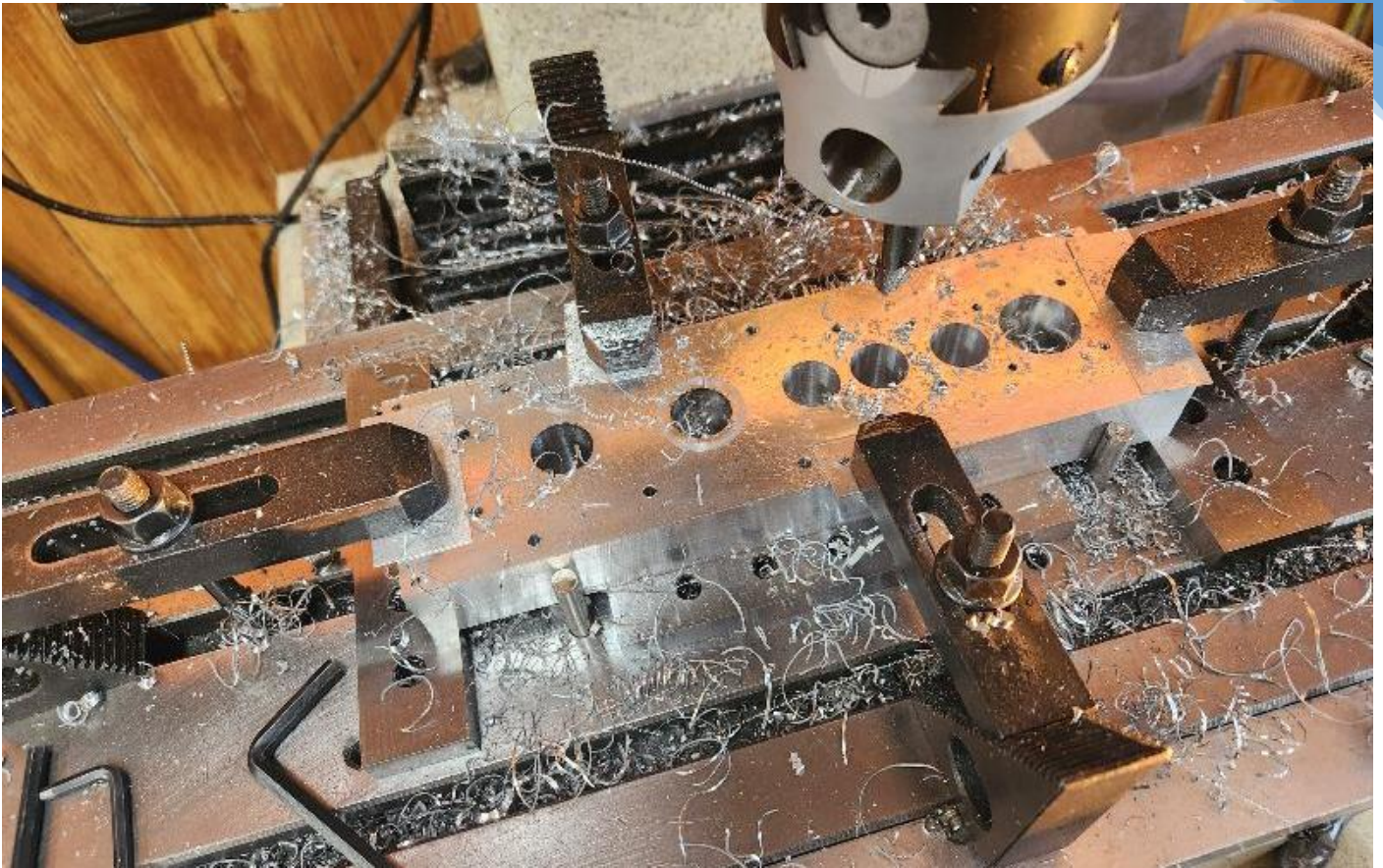
Above; Boring bearing holes. Right; broaching tool
