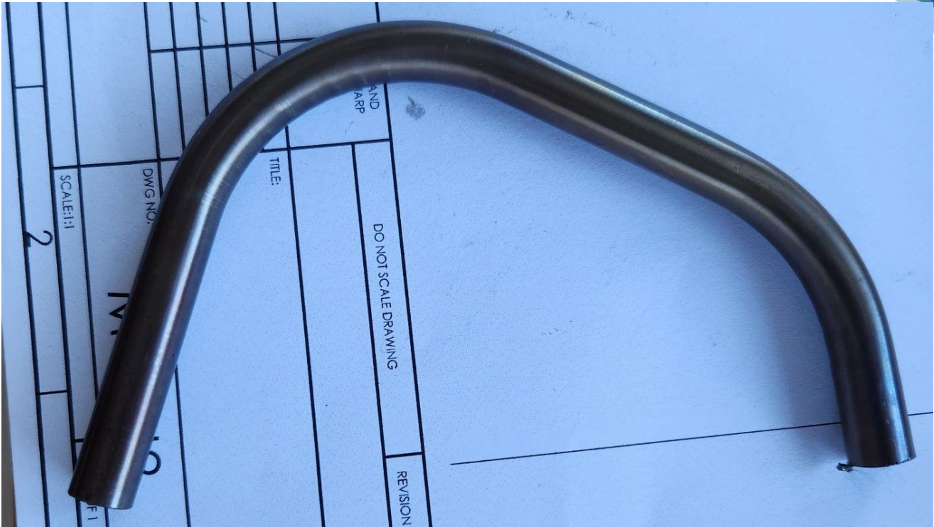
Pipe bend. A better bend, I filled the pipe with lead and melted it out after. Works great!
