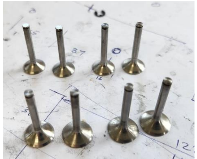
Right; Completed valves, one spare!
