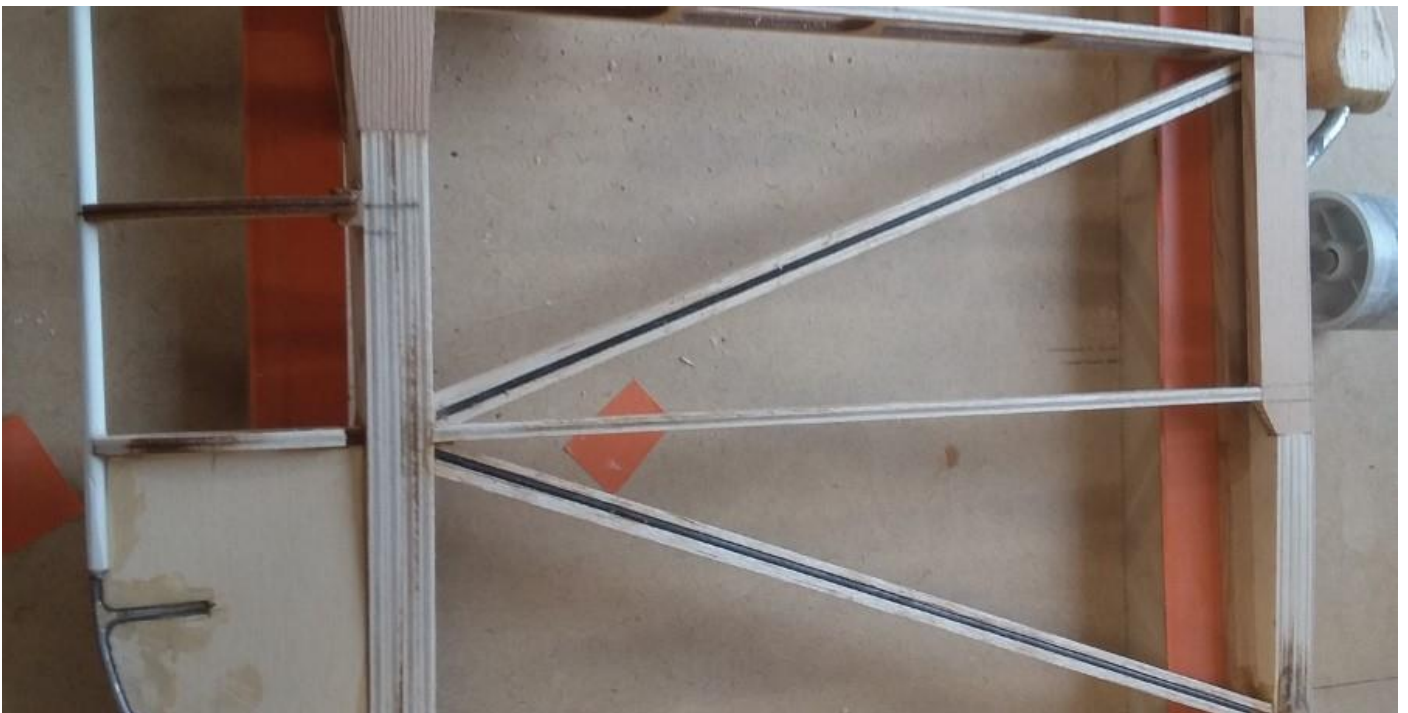
Above; Carbon reinforced wing bracing.
