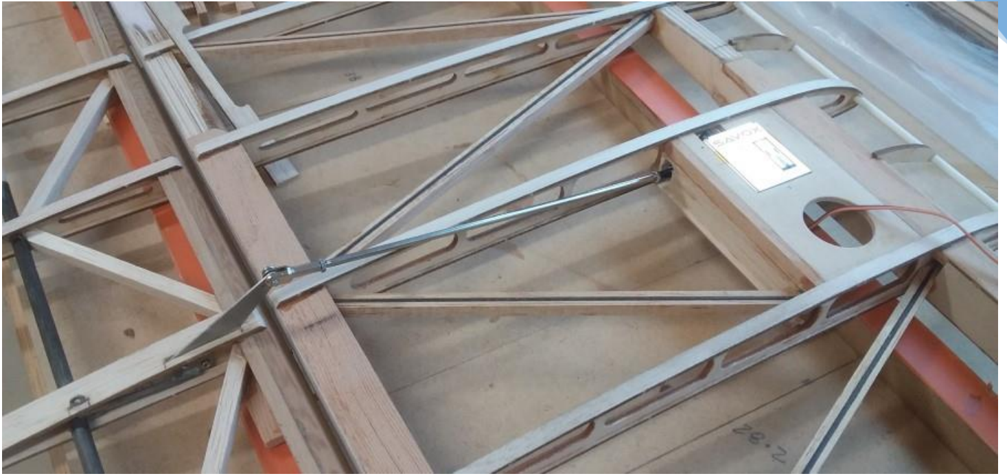
Above; Aileron linkage and servo (Savox wing servos 8kg.)
