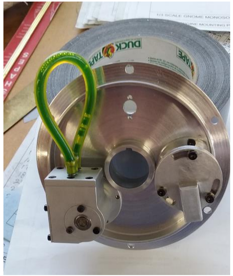
Right; Mounted oil pump and ignition pick up.
