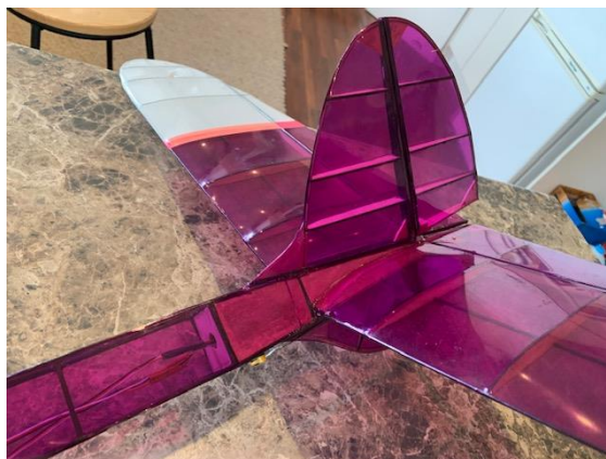
Left, Pete T with his Civvy Boy, and Right, the rear end of Pete’s E Rubber model “Rocket” showing his all carbon sq/tube construction for a very rigid and light aircraft.
