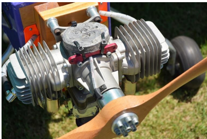
111cc Twin power plant fronting the the Stik.
