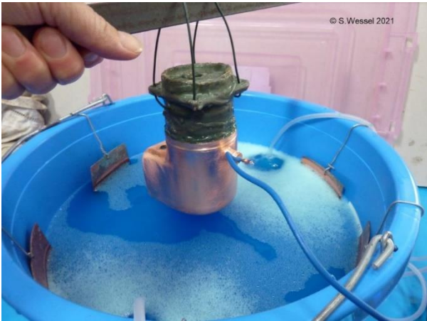
Left; Electroforming Jackets.
