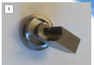
Seen here in pics #1 through to #4 is the progression of Phil's work in constructing the Valve Cage / Cylinder heads. (9x !!) Fig 1 starting with a round billet of steel, all he had available, band sawing it a rectangular block. Milling the side flutes and then using his 4 jaw chuck (He tells me !) turning up the head and valve seat. Figs 2 & 3..
