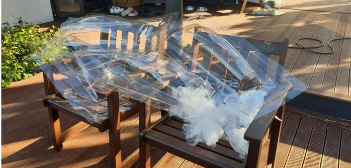
We decided to have a go at vacuum forming the canopy so made a buck (Plug?) from plaster of paris, built a rig and sourced some plastic. We have used the BBQ and a heat gun, two old vacuums and some MDF. After some failures (learnings!) we finally got a useable canopy. Small parts are a piece of cake but the larger canopy was challenging - we will try some wheel pants next.
