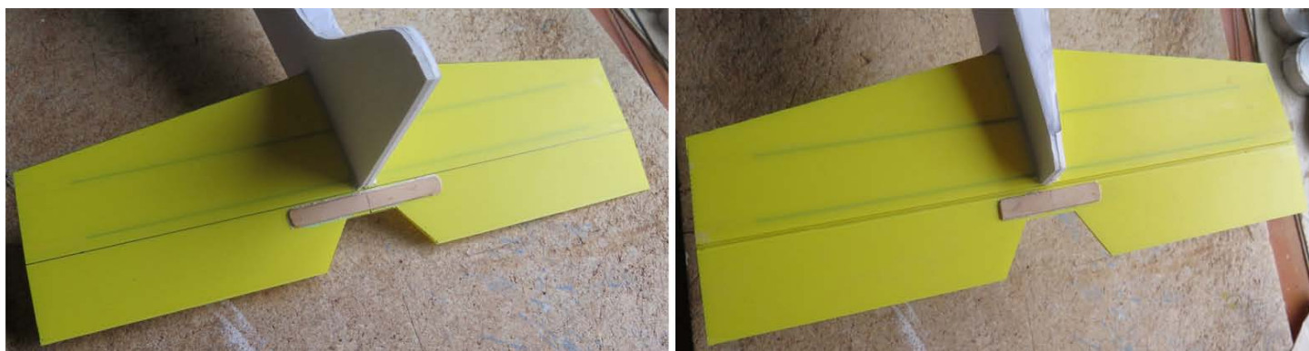
Fig 5 The coreflute elevator with carbon stiffening rod, ply joiner and epoxied into fuselage slot.
