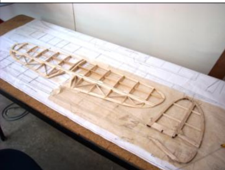
The tail surfaces all done and the rudder all glued up
