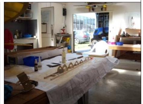
The fuselage spine frame set out and glued.
