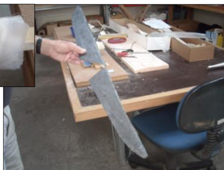
Some carbon fibre tissue epoxied to the underside of the elevator - cut out the open parts to give strength.
