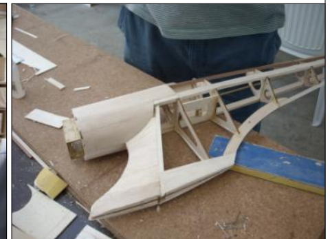
Front sheeting almost done.
