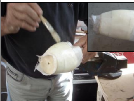
Barrie fibreglassing the foam nosecone mould.
