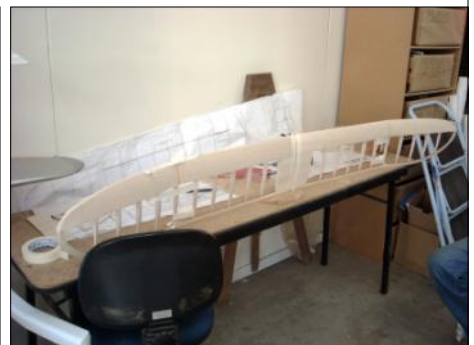
Wing, and all the polyhedral epoxied up drying.
