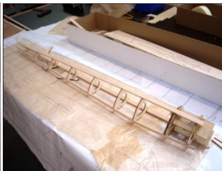
The fuselage bottom and motor mount
