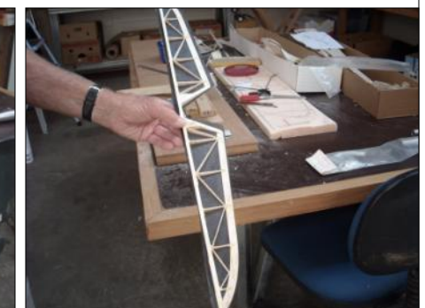
Some carbon fibre tissue epoxied to the underside of the elevator - cut out the open parts to give strength.
