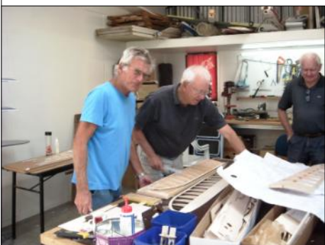
Stan and Barrie putting wing cap strips on
