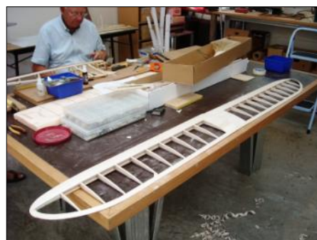
The almost complete wings all ready for dihedral.
