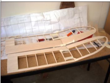
Two wing halves all glued and taped.
