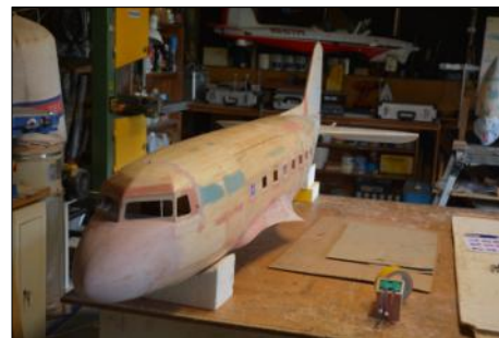
Fuselage front all filled and sanded.
