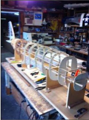
Framing up the fuselage
