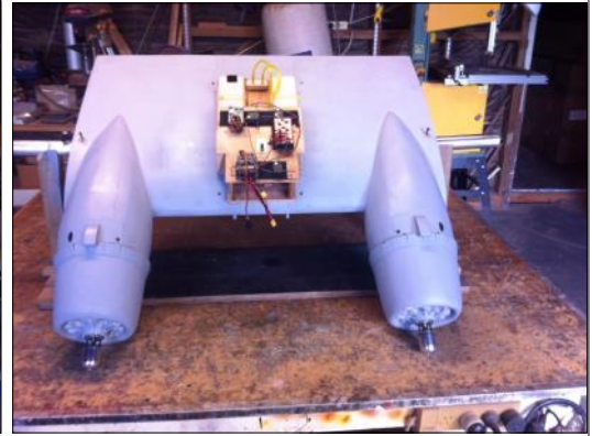
Engine centre section with nacelles and cowlings
