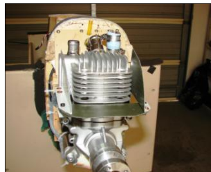
More 'front end' cowl and engine cooling modifications
