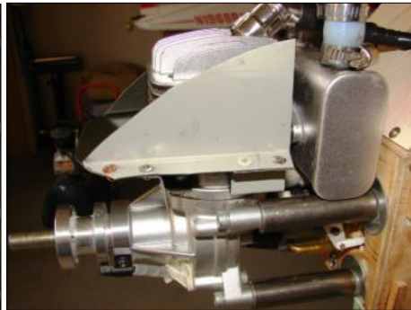
Cowl and engine cooling modifications
