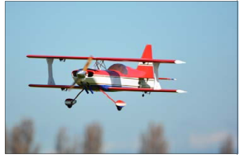
The Mike Shear's aerobatic Biplane also got its first outing and maiden flight. Needed a good bit of nose weight after the maiden flight to get it into trim, but otherwise test pilot Jayden Molloy and Mike Shears seemed well pleased with the model after several flights on the day.
