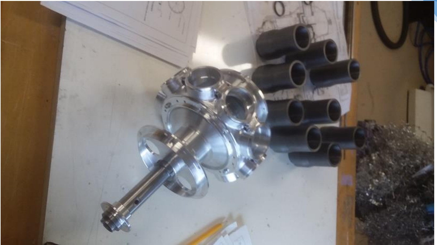
Crankcase with crankshaft in situ with rear mounting plates in place. Nine cylinders shaped and bored ready to go to be honed to the correct size. The thinner bottom end locates in the crankshaft and the tapered thicker top end has the cooling fins cut into.
