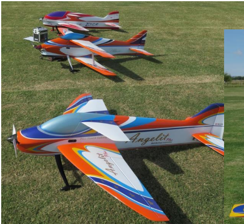
Above, electric powered Pattern aircraft, amazing 2 metre models weighing under 5 kg fully loaded with 10S 5000+ battery packs ! I'll accept the fact they look like flying fish, but it's a pity they don't sound like "real" aeroplanes !! ( sob, tears....just jealous !)
