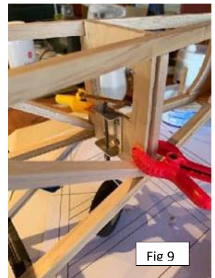
Fig 9 Tailwheel mounted on lite-ply and temporarily clamped in position. Fig 10 Tailwheel assembly set aside for now and it's back to the wing mounting above the cabin. Using hardwood the wing mount above the cabin top is mortised and glued with a diagonal support to the top longeron. The dark spot at the joint is a treenail, or tree-nail (as used in boat building) where a hole is drilled and a glued wooden nail—in this case a length of bamboo skewer—makes a tight fit to secure the joint. The diagonal is also fixed to the top longeron with a treenail. Fig 11. Stringers fixed to the underside, with motor in place F1 is positioned and glued
