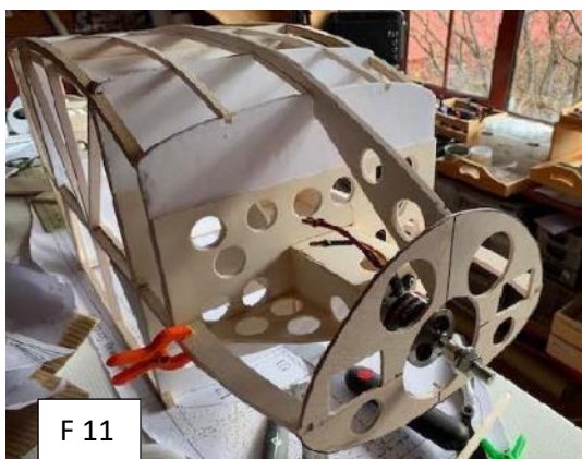
Fig 9 Tailwheel mounted on lite-ply and temporarily clamped in position. Fig 10 Tailwheel assembly set aside for now and it's back to the wing mounting above the cabin. Using hardwood the wing mount above the cabin top is mortised and glued with a diagonal support to the top longeron. The dark spot at the joint is a treenail, or tree-nail (as used in boat building) where a hole is drilled and a glued wooden nail—in this case a length of bamboo skewer—makes a tight fit to secure the joint. The diagonal is also fixed to the top longeron with a treenail. Fig 11. Stringers fixed to the underside, with motor in place F1 is positioned and glued
