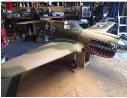
It is powered with a DLE 55 and steered by Spektrum. Maiden flights are now due and will take place when the field is open. Set up flights will be done and checked, then then a repaint job in RNZAF colours will follow. I have really enjoyed doing this model and it's a sad day that the manufacturer terminated production on these.
