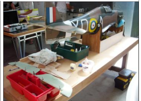
The Hurricane gets its elevator hinged.
