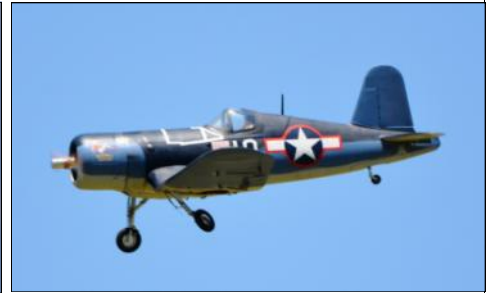
On approach with the port gear Not down and locked.
