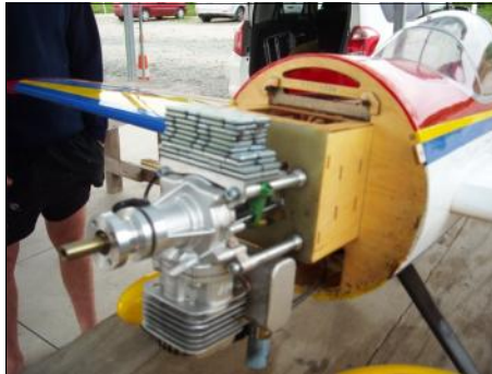
And, No the layers Above the engine are Not another engine cylinder - just some lead weight to get the C/G. forward. Mike Shears and Alex Wardley offer their advice.
