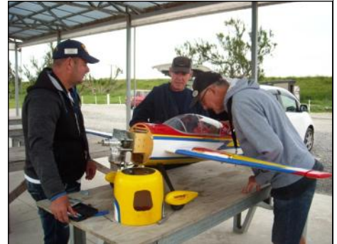
And, No the layers Above the engine are Not another engine cylinder - just some lead weight to get the C/G. forward. Mike Shears and Alex Wardley offer their advice.
