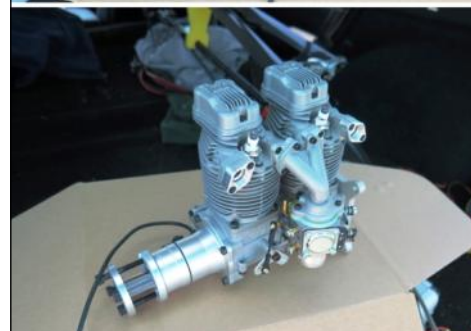
Phil Sharp's new 60cc NGH in line twin FS
