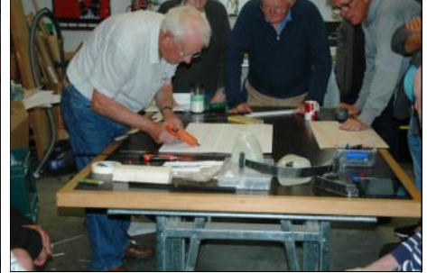
Gluing the spars in with hot glue.
