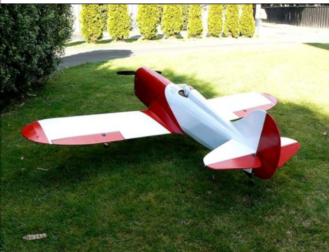
GEE BEE 90% finished, has flown. 1.96m (77") wing span, DLE 20cc
