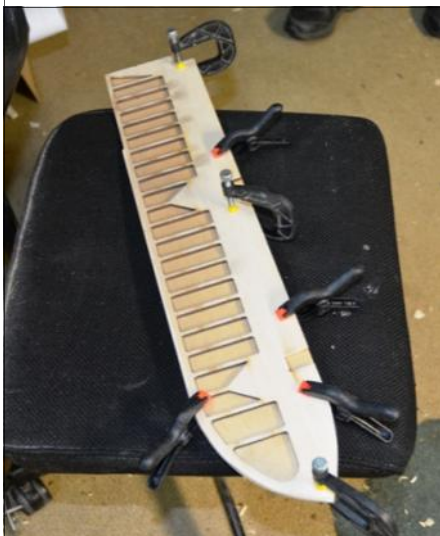
Aileron construction - to be skinned top & bottom.
