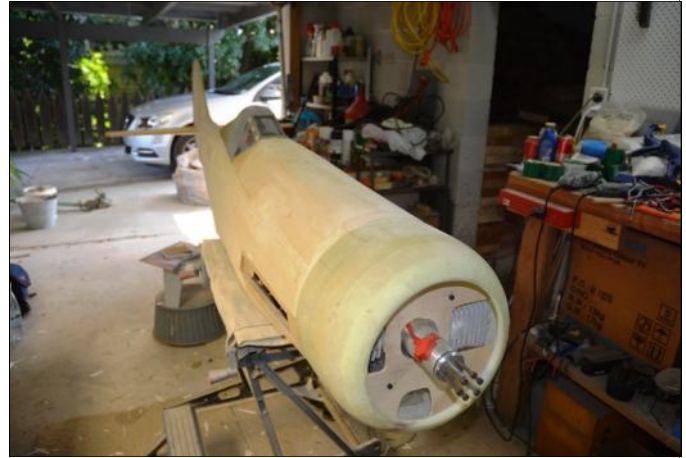
Fuselage now almost done, cockpit completed, engine installed and cowling made. Working exhausts yet to be constructed.
