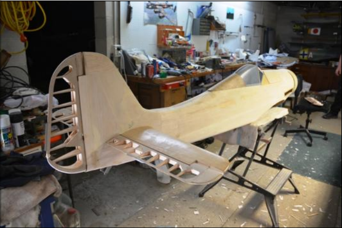
Fuselage now almost done, cockpit completed, engine installed and cowling made. Working exhausts yet to be constructed.
