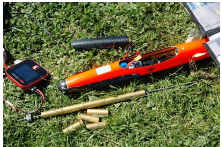
The front end of a well dressed F5J electric model - showing ballast too.
