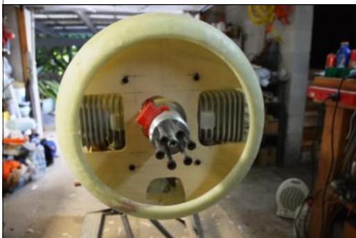
The front end - with cowl on and off. Power is a 100cc twin!!!
