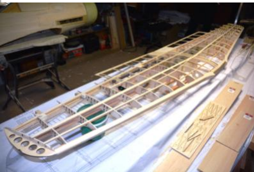
Wing construction in all its glory! Light but strong.
