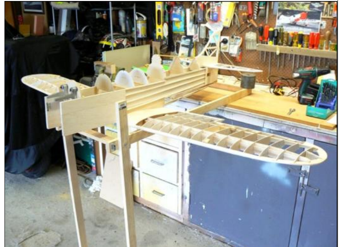
GEE BEE Model 'D' Sportster under construction
