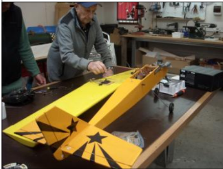
Kevin's trainer model having the aileron servos changed .
