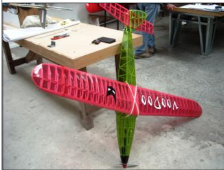
Some other views of the very lightweight structure and controls...
