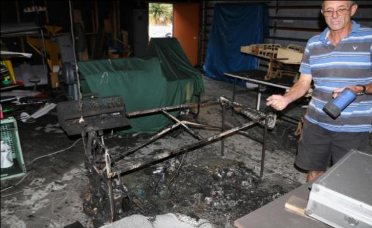
Hamilton modeller's workshop after a fire from charging a 3 cell 2200mah lipo battery. The heat and the contaminants from this fire totally destroyed or rendered useless everything inside and including the shed
