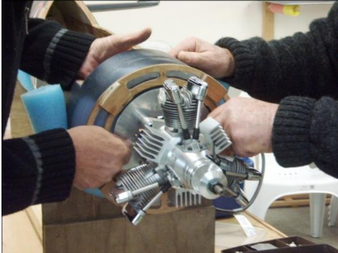
The 3 cylinder Saito 'beastie' being mounted in place.
