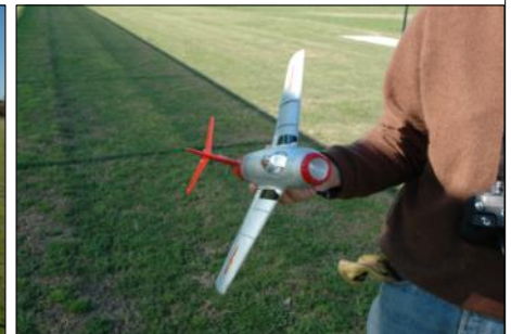
Jerry's tiny Mig-15 electric. Has rudder, elevator, throttle and ailerons!
