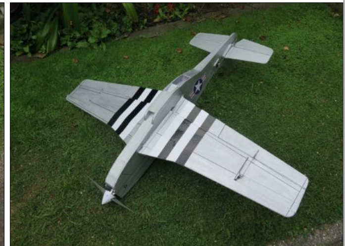
Painted with a test pot of Resene silver acrylic paint, some vinyl markings and a waterproof pen panel lines.
