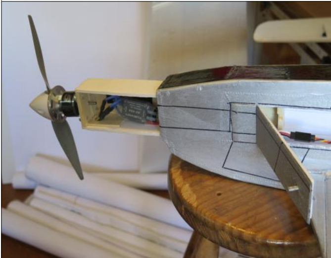
Motor power pod sliding in and the battery access hatch.
