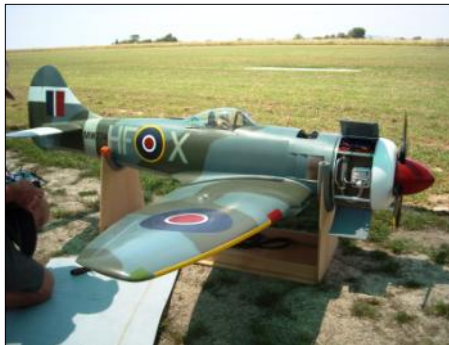
The Tempest engine internals (DA100cc twin)
