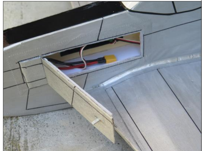
Motor power pod sliding in and the battery access hatch.
