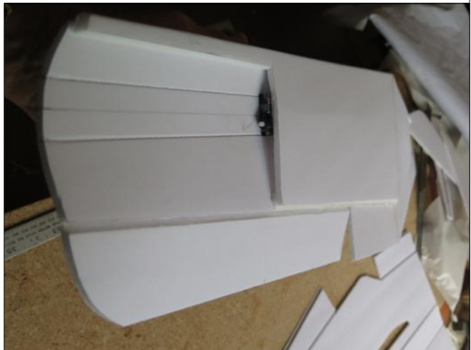
Mustang fuselage foam sheet ready to fold and glue & Wing half folded and hot glued.
