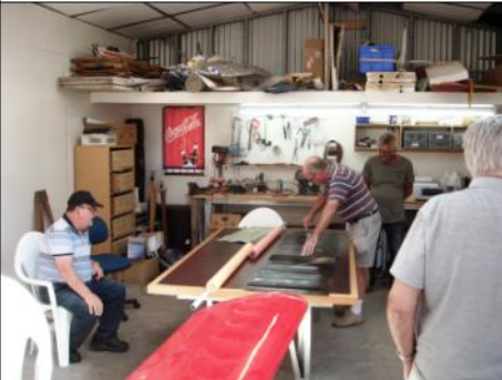
Phil Sharp brushing on contact glue to the rubber sheet.
