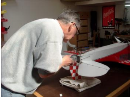
Mike Shears making some elevator hinge slots
