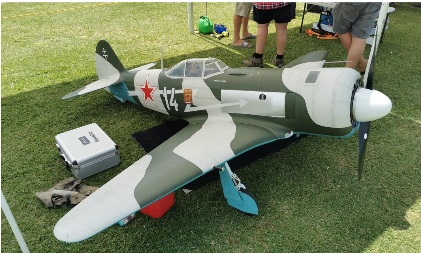
This one third scale Yak 11 from a German Airworld ARF kit, with exceptional detail finish is co-owned and campaigned by Grant Plaisted and Carl Hansen . Powered by a 5 cylinder Moki 300 engine it looks and sounds magnificent in the air.
