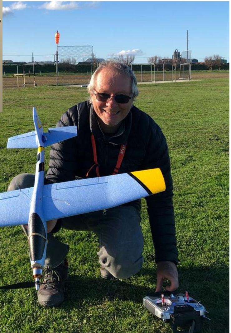
*solid and light. I hollowed out the fuse from the nose to the wing saddle allowing the receiver and esc to sit in the front wing saddle — to get CG. CG is set at 55mm but I think that 60mm would be even better. I have not moved the wing and in this scenario 60mm would set better I think. Easy to experiment.*
