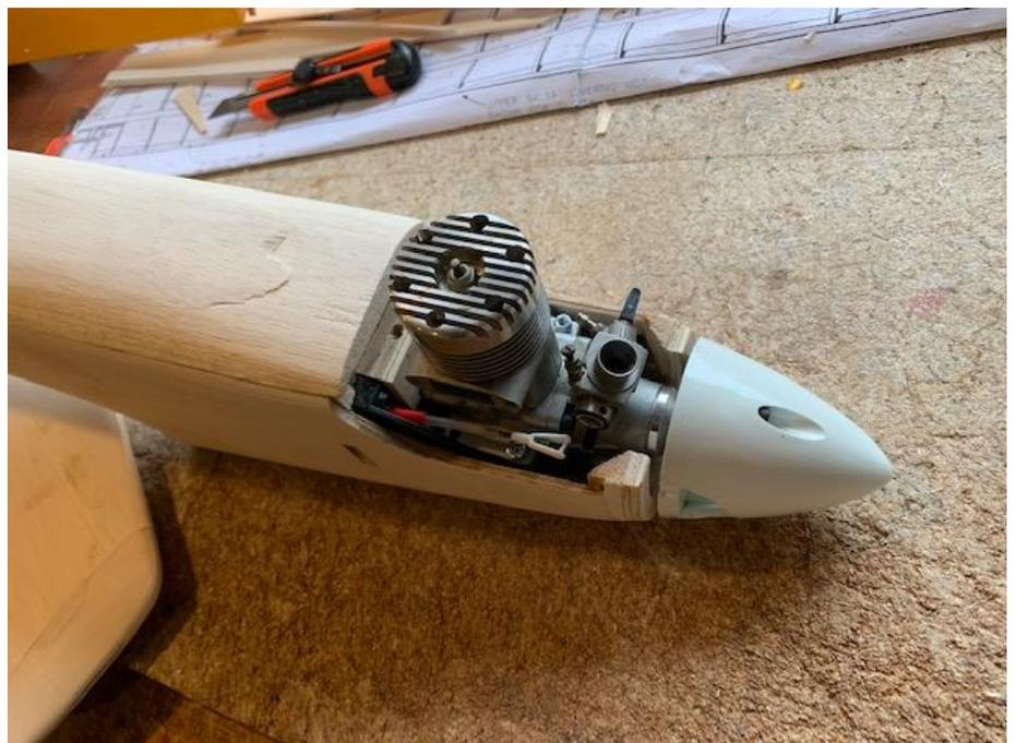
The last job is glassing the fuselage for a more durable paint finish and the tail and flying surfaces are covered in shrink film. On the fuz I've epoxied on a fine 1.4 ounce glass cloth and when finished will be sprayed with a one step filler primer and well w/d sanded to a fine finish. The finishing paint will be base coat white and a two pot clear glossy top coat.
