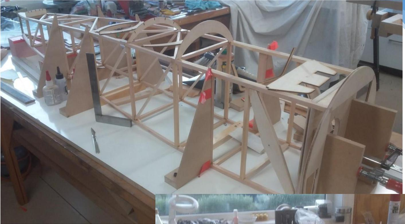
I asked **Phil** about his gluing regime, He uses mainly Titebond pva for the wood frame joints and will be adding a fair amount of gusset for strengthening. Around bulkheads and the firewall etc he uses an epoxy adhesive for extra strength.
